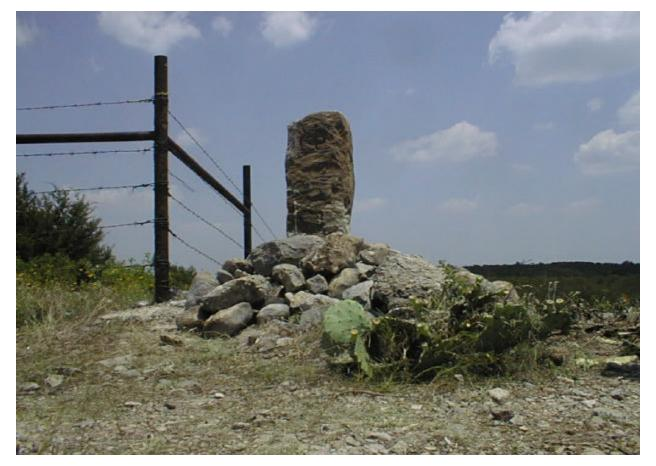
"Set Sandstone 54 x 18 x 18. Marked on West side I.P. on East side Ind. Mer. on North side 1870, in a mound of stones 6 feet in diameter and 3 feet high from which Flagstaff at Fort Arbuckle bears N07°37'W..."
